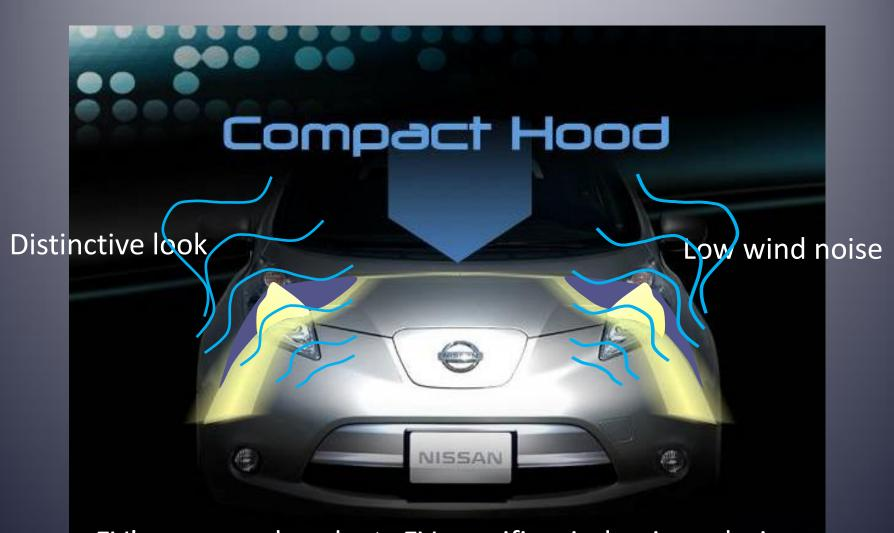
EV's compact hood ⇒ EV specific wind noise solution Also good for Aerodynamics
